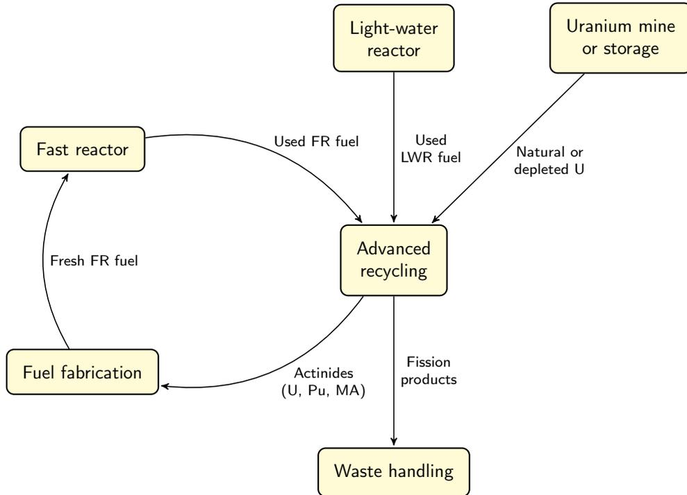
Figure 1: Some advanced recycling techniques allow for repeated recycling of fuel for fast reactors, with all actinides extracted as a group.
