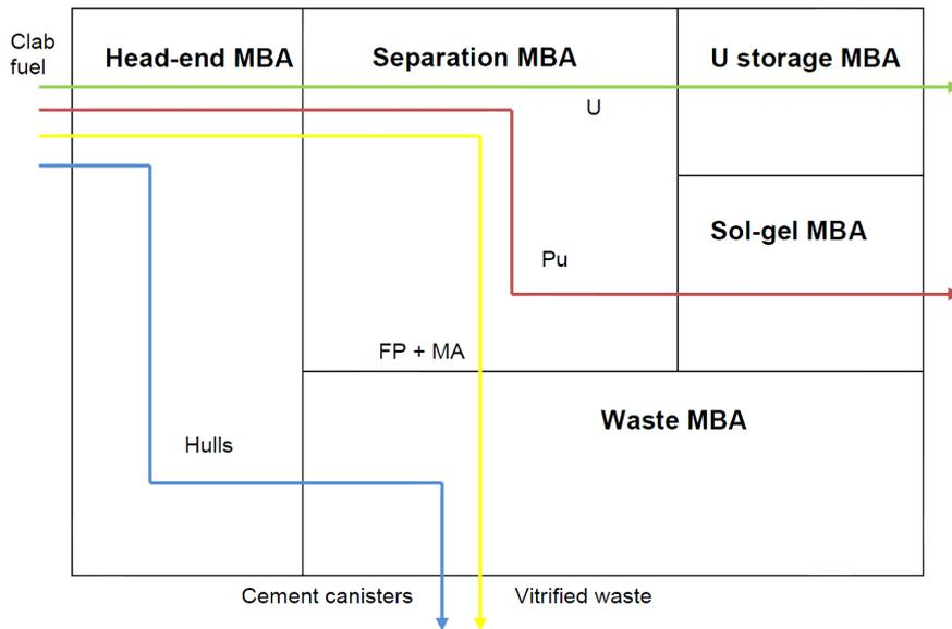
Figure 2: Schematic design of the recycling in Electra CC, Phase I. In the Head-end MBA, used fuel is received and dissolved as a preparation for the separation process. In the Sol-gel MBA, the solution containing separated Pu is manufactured into microspheres in a sol-gel microsphere pelletization process.
