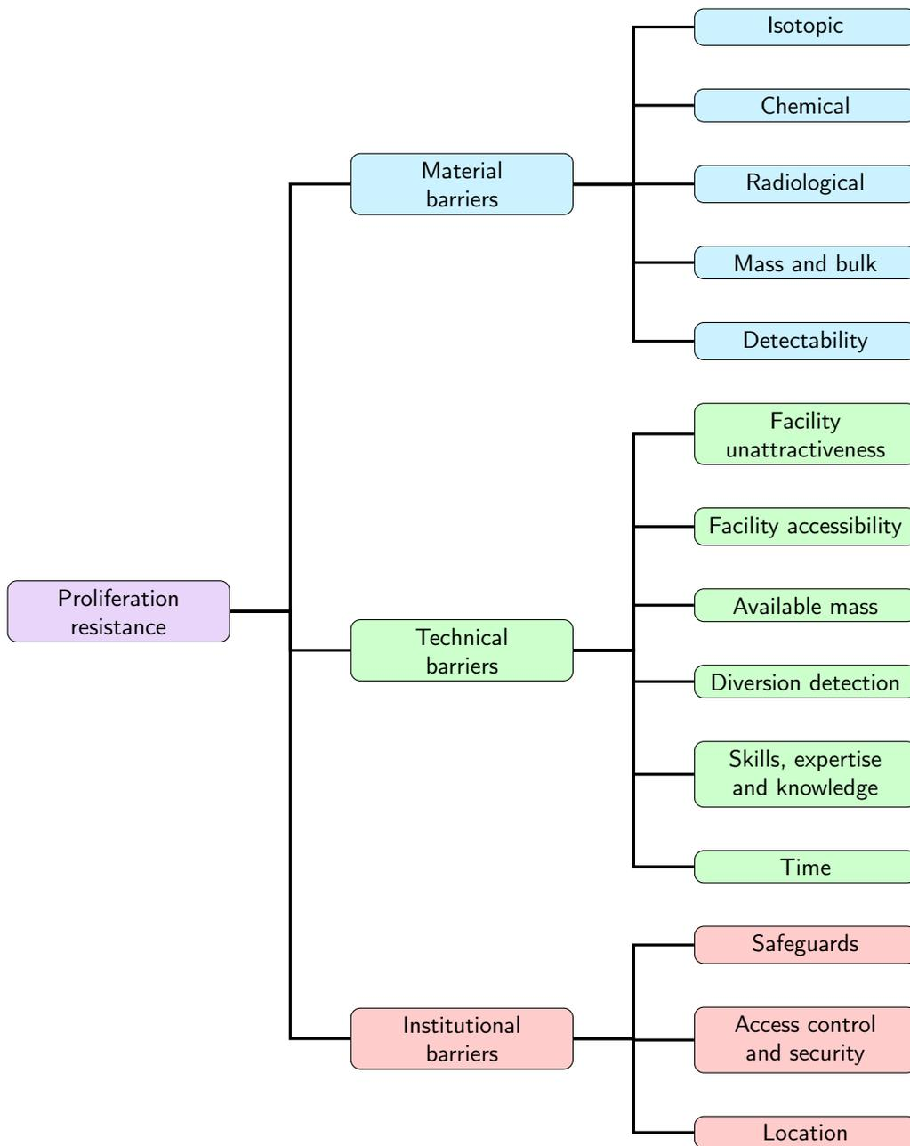
Figure 3: Graphical overview of the TOPS methodology illustrating how the total resistance (left) is estimated based on the barrier categories (center) and barriers (right).
