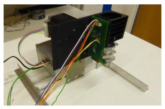
Figure 3. Star tracker of motorized rig.
