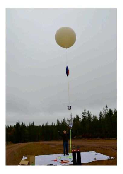
**Figure 1:** The moment of launch - Henrik Åkerstedt from Vetenskapens Hus prepares to release the balloon. The lower white polystyrene box contains the cosmic-ray detector and cameras. The upper box contains the radio equipment and weather sensors. The parachute can be seen in the line connecting the balloon to the payload boxes.
