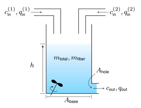
A tank is being filled by a mixture of fiber and water
