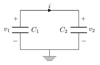
Can we compute the current i flowing through the capacitors?
