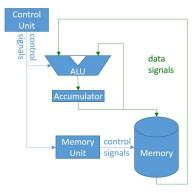
**Figure 4: Accumulator Architecture**
