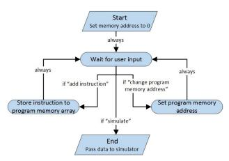
**Figure 2: Programmer State Machine**
