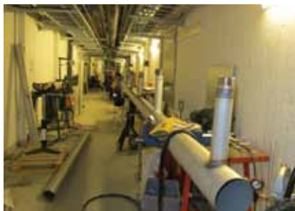
Above: The basement of PDC was used as a workshop to produce the necessary cooling pipes.
