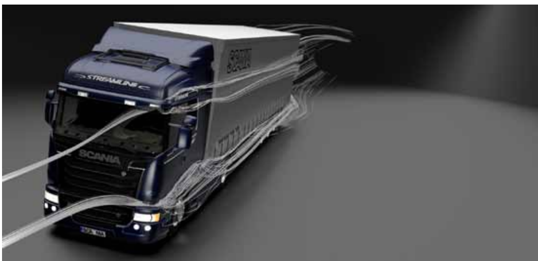
Above: Results from an aerodynamic simulation showing streamlines around a Scania truck equipped with a trailer
