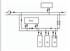
Ring shaped cooling system at the campus. The check valve closes and a self-supplying section is formed once building 19 (the Chemistry building) is capable of taking care of all waste heat in the section. This happens at about o °C outdoor temperature. PDC uses coolant from both sides of the check valve.
