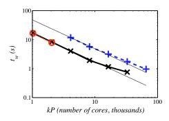
Figure 3: Wall time per time step for a fixed problem size (strong scaling) as a function of number of cores on Cray XE6, PDC (×), Blue Gene/P, ANL (+) and the AMD Opteron cluster Ekman, PDC (o). Ideal scaling is included for reference (solid line). Simulation performed by Ohlsson et al., 2010.
