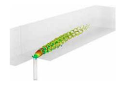
(d) Vortical structures in a jet-in-crossflow with a mesh including a flush-mounted pipe. This case consists of a jet of fluid exiting a nozzle and interacting with the surrounding fluid. It is a flow of high practical relevance with a number of applications like smoke and pollutant plumes, fuel injection and mixing or film cooling (Figure by Adam Peplinski).
