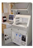
The capillary electrophoresis instrument (left) registers spectrums of fluorescent labelled DNA (middle), which are analyzed at the laboratory and thereafter transmitted to PDC for permanent warehousing.
