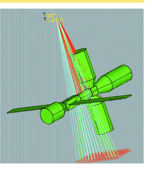
Fig. 1 A point source is situated above a generic satellite. The shortest direct and reflected path between the source, indicated by the yellow coordinate system, and the observer points underneath the satellite are searched for in the ray tracer. The direct and the reflected GTD (Geometrical Theory of Diffraction) fields are summed up at the observer points. Green rays follow the reflected field, blue the direct, and the red rays indicate occulted direct rays.
