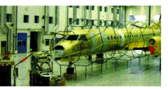
The compatibility of electromagnetic devices is currently an impor tant issue in the automotive and aviation industries. The EMCP2 project has resulted in a method whereby the placement and interaction of electromagnetic devices can be optimized using computer simulations and then validated using measurements.
