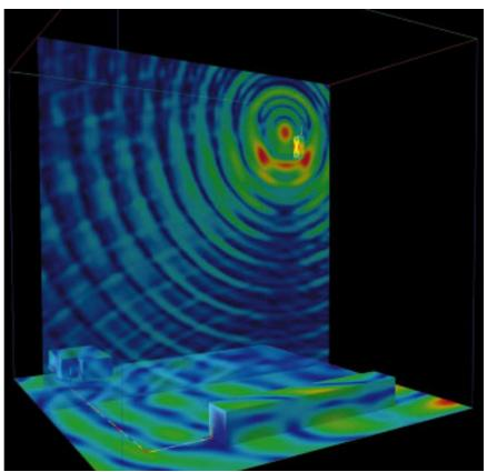
A model setup for studying the induction of currents on a wire connecting two electronic devices in the presence of a transmitting cellular phone. The antenna on top of the telephone is driven by a current pulse and the picture shows a snapshot in time of the response. Execution time on the Fujutsi VX/2 at PDC was a few minutes and execution speed almost 900 MFlop/s.
