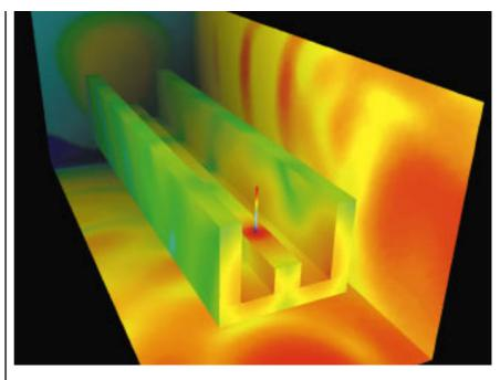
This figure shows, for a distinct time, the solution of an open waveguide problem. An antenna is attached to an E-shaped waveguide and a current pulse is injected into the antenna.
