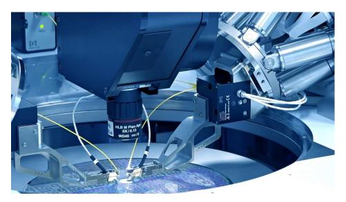
Figure 1. Measurement concept for CMOS circuit testing with quantum sensors: a microscope objective collects infrared light emitted by an integrated circuit under test. This allows for new studies of the circuits performances.
