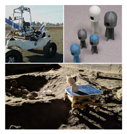
Figure 1.1: Left: Picture of our KREX-2 rover with the SPEARS launcher mounted on the front. Right: A family of SPEARS projectiles. Bottom: Mock-up of a rover parked at the edge of a crater with the projectile sensor from Chapter 6 deployed to the centre.
