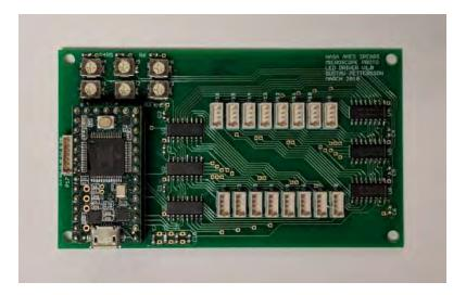
Figure 3.3: Control electronics for the microscope.
