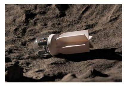
Figure 6.1: Deployed projectile mock-up microscope.
