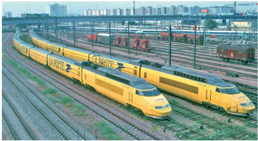
The French TGV postaux – with a maximum speed of 270 km/h – are the fastest freight trains in the world today.
