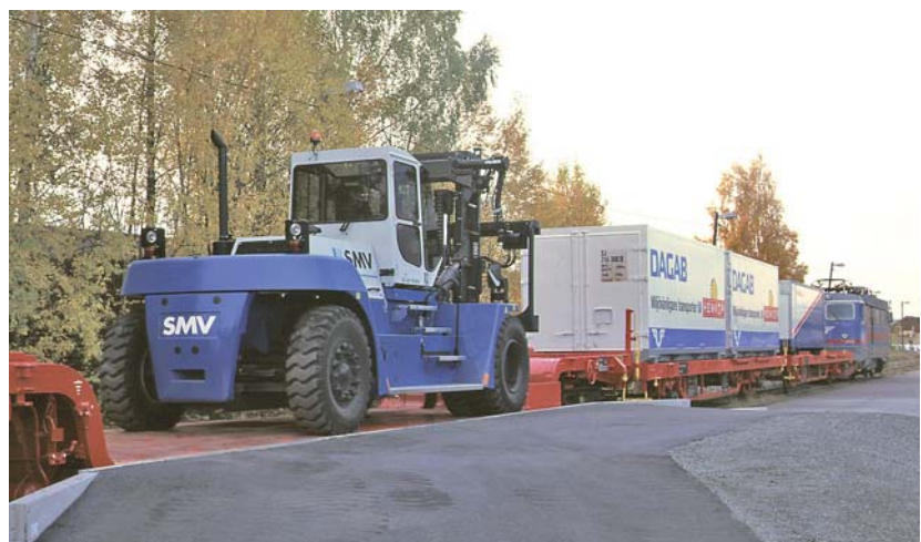
With a “Light-Combi” system the railway can be competitive for smaller consignments of high-value goods over shorter distances. The picture shows the Swedish experimental train where a fork-lift carried on the train and operated by the driver, unloaded and loaded swap-bodies under the catenary at small terminals along the line.
