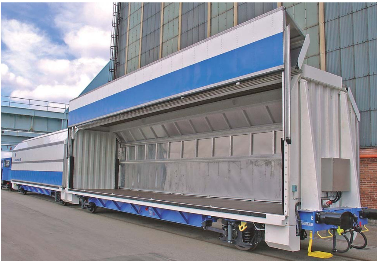
"The Europe-wagon" made by K-industries is a large-volume wagon with a low floor, a substantial loading area, and track-friendly running gear.
