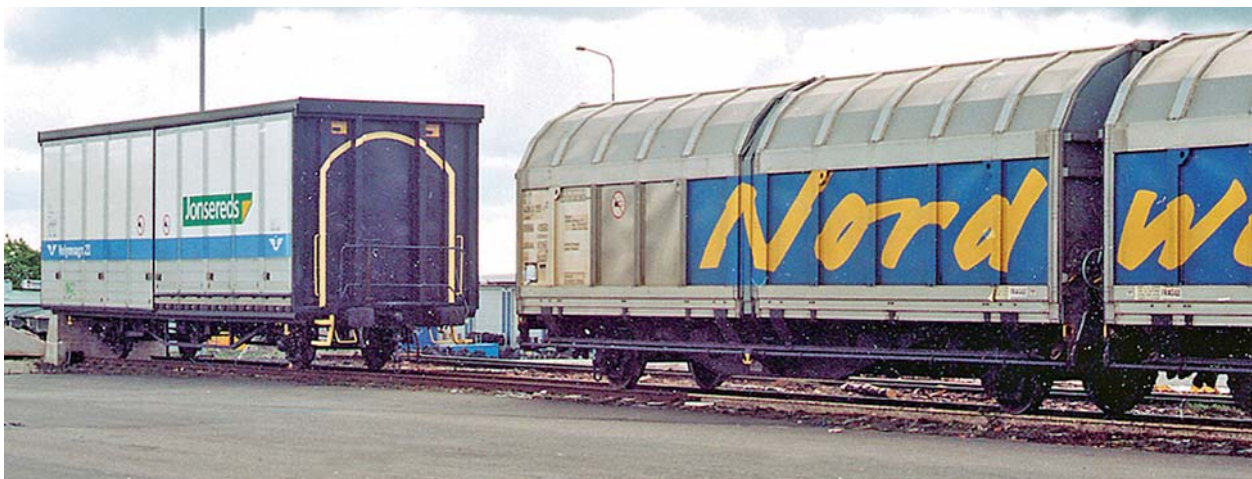
A wider, square-shaped loading gauge instead of the one with rounded corners currently in use is an important factor in reducing the transportation cost of volume freight. The illustration shows a C loading gauge wagon in comparison with the normal G1 loading gauge.
