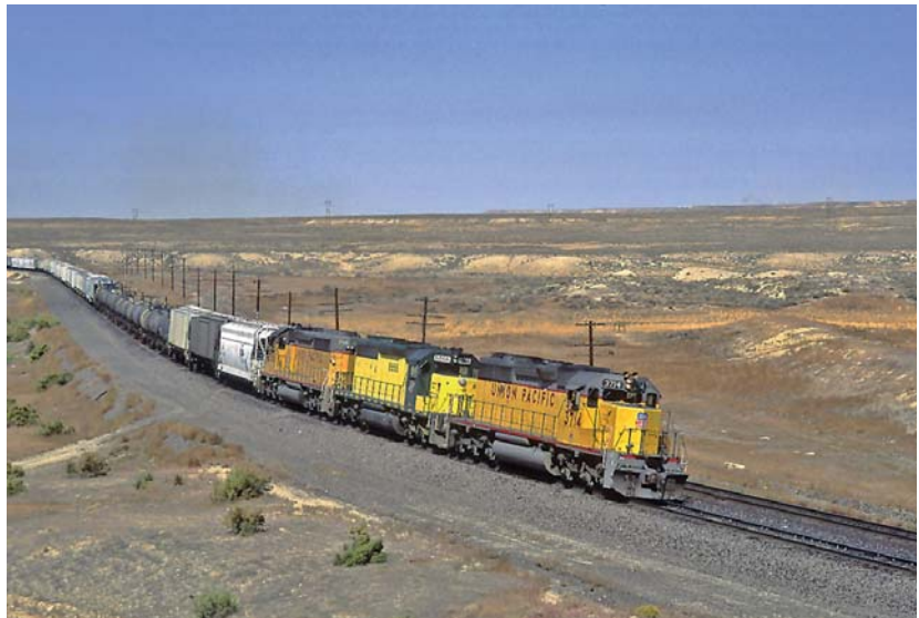
Freight trains in the USA can be 2-3 km long with a gross weight of 10,000–15,000 tonnes. They have automatic couplers and generally more than one locomotive.
