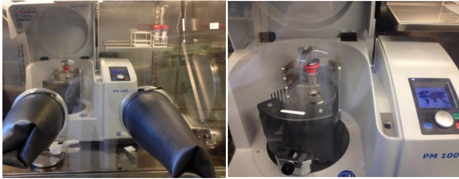
Figure 10: Retsch PM 100 in a glovebox used for milling
