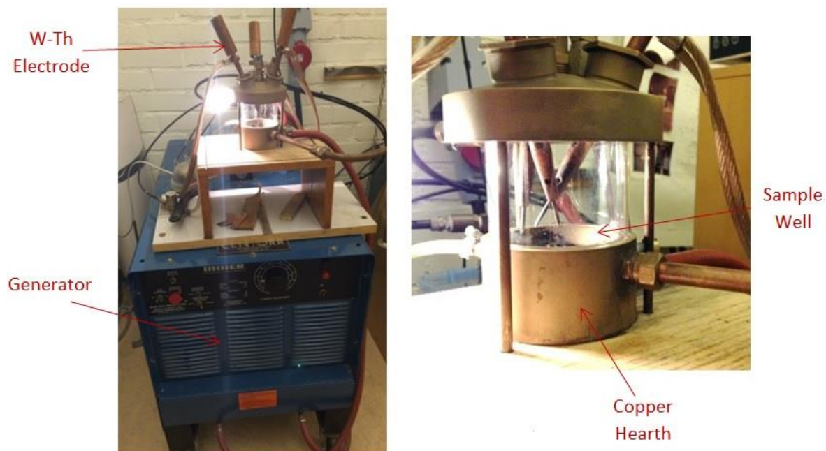
Figure 9: Arc melter used for melting the alloys
