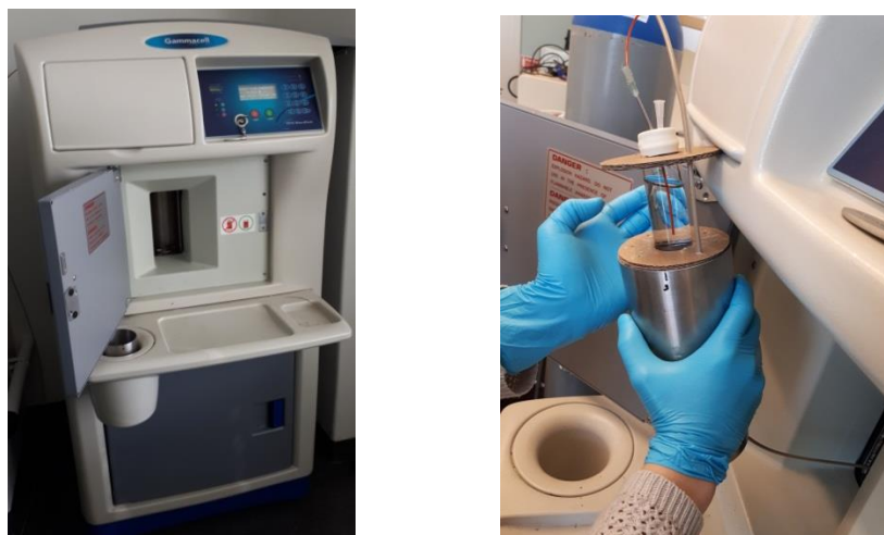
Figure 13: Gammacell 1000 Elite MDS Nordion (left) and the experimentation set-up (right)
