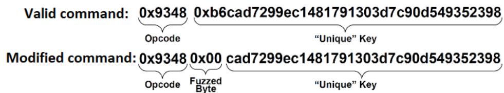
Figure 2.6: Inserting a fuzzed byte into a valid command[28].
