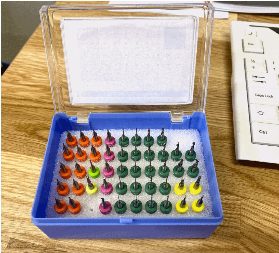
Figure 19: The tools available for use for the PCB mill in the student workshop
