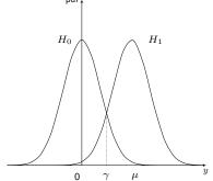
The intersection point of the two adjacent gaussian curves defines the threshold  $\gamma$ , according to which a decision is made
