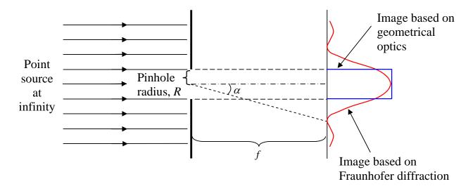
The image of a point object, the Point Spread Function (PSF), should be as small as possible to produce a sharp image.
