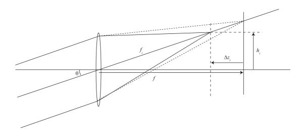
Finally, we try to find and plot the tangential and sagittal focal planes. Start at the paraxial image plane and measure the focal length f. Then use a field angle  $\theta$  of  $10^{\circ}$ ,  $20^{\circ}$ , and  $30^{\circ}$ .
