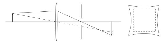
Build a set-up to view pincushion distortion. The object is a piece of an OH sheet with millimeter markings, and you can use the largest of the metal pinholes as aperture. Remember, the object must be diffusing but the aperture must not! Use a lens of focal length  $50 \, \mathrm{mm}$ . Study the effect of moving the aperture and write down your findings.
