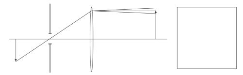
Use a large-aperture 200 mm lens (without iris diaphragm) to image a pinhole (use the one with multiple holes, as those are the smallest) onto the screen. Use another aperture, either the largest metal aperture or one made of paper, to force the rays to pass close to the edge of the lens. Adjust your set-up until you can observe lateral chromatic aberration. **Draw a figure of the image in the box above!**
