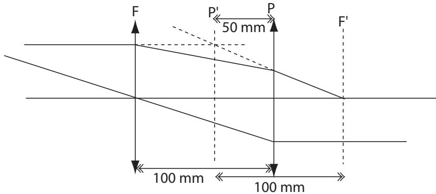
$W_{222})/H^2 = -\frac{11}{3}(K_1 + K_2) = -55 \text{ m}^{-1}$  and  $r_t = -18 \text{ mm}$ . These are steep curvatures! (The expressions for the curvatures could also be derived from the longitudinal aberration and the sag formula.)
