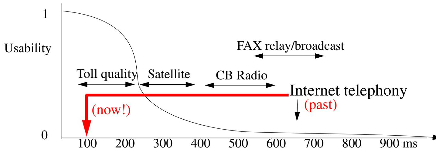
Figure 2: Usability of a voice circuit as a function of end-to-end delay (adapted from a drawing by Cisco<sup>a</sup>)
