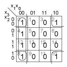
$$f = \overline{x_1} \overline{x_0} + \overline{x_2} \overline{x_0}$$
