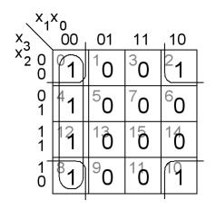
$$f = \overline{x_1} \overline{x_0} + \overline{x_2} \overline{x_0}$$
