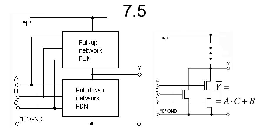
Pull-down circuit is the inverted function. The Pull-up circuit is the function noninverted:
