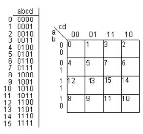
The frames are ordered in such way that only one bit changes between two vertical frames or horisontal frames. This order is called Gray code.
