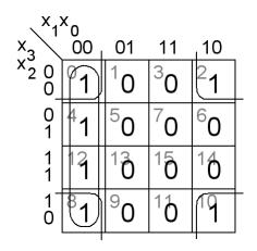
$$f = \overline{x_1} \overline{x_0} + \overline{x_2} \overline{x_0}$$
