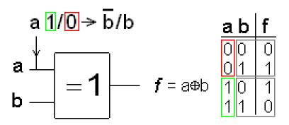
When the control signal is a "1" the gates output is b's inverse, when a is "0", the output is equal to b
