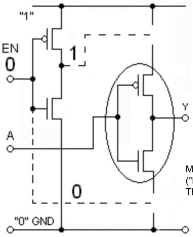
When EN = 0 the output is totaly disconnected from the supply voltage and ground. A can no longer influence the output value.
