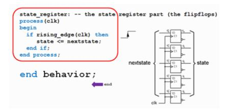
By using the function rising\_edge(clk) we let the compiler "understand" that we want to use the flip-flops inside the MAX-chip in order to build a register.
