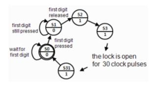
The Code Lock template applies to a simplified lock that opens when you press the key "1" and then release the key.
