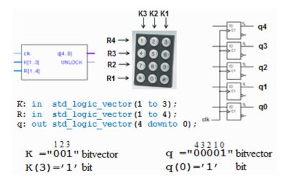
You can customize the indexing of variables so that it is consistent with the data sheets - less risk of mistakes!
