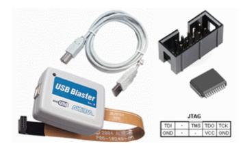
Connect the USB blaster to your computer. Connect the USB Blastern JTAG connector to lab equipment. Note! The lab equipment's voltage shall be off when plugging in or unplugging the JTAG connector. Lab equipment's voltage must be turned on when you program the chip-USB power alone is not enough for this.
