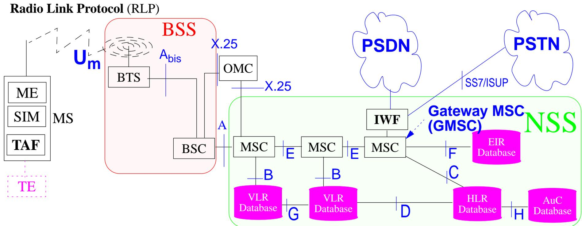
Figure 25: GSM/HSCSD Architecture
