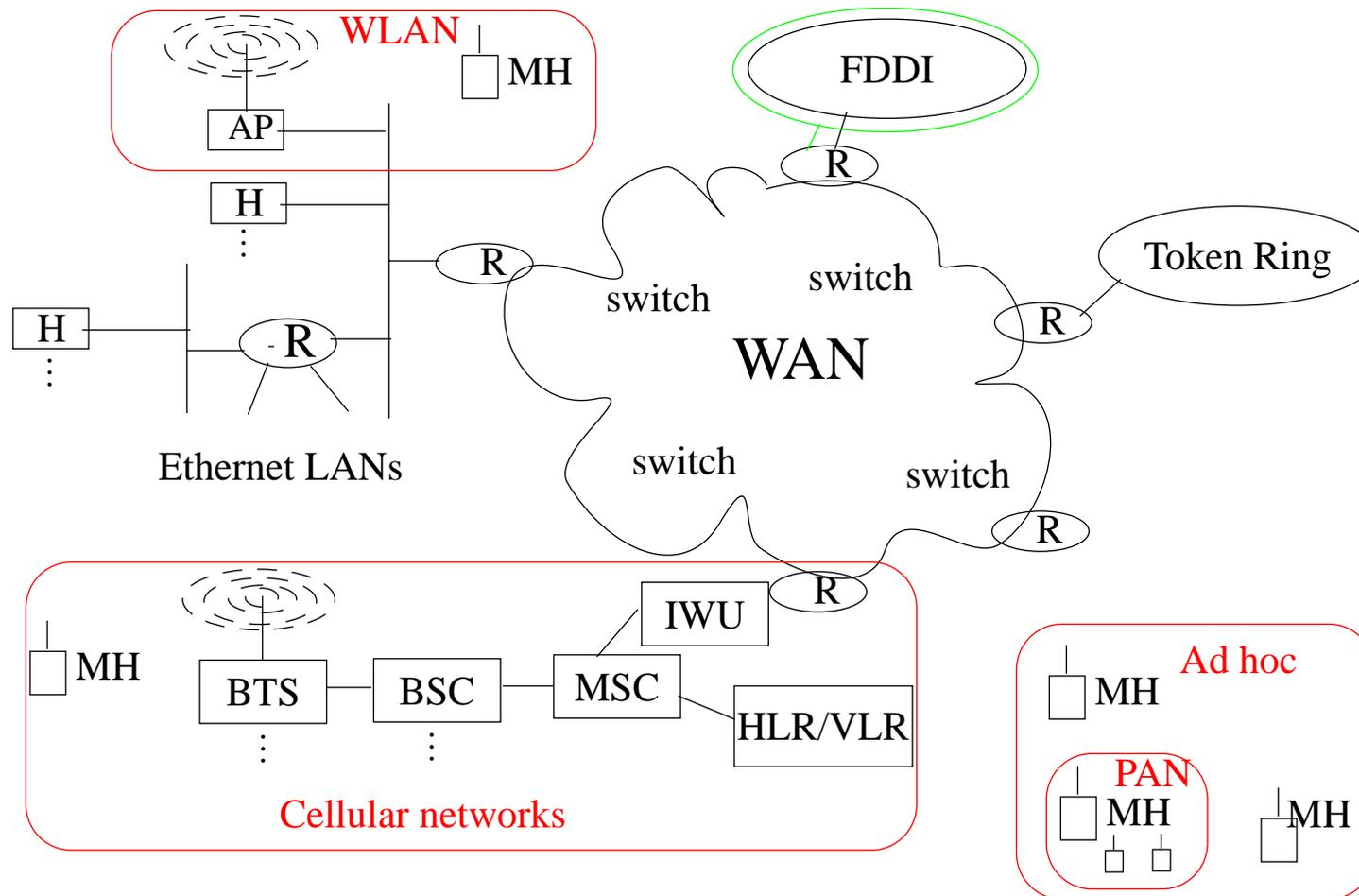
Figure 1: Multiple network technologies - *internetworked* together
