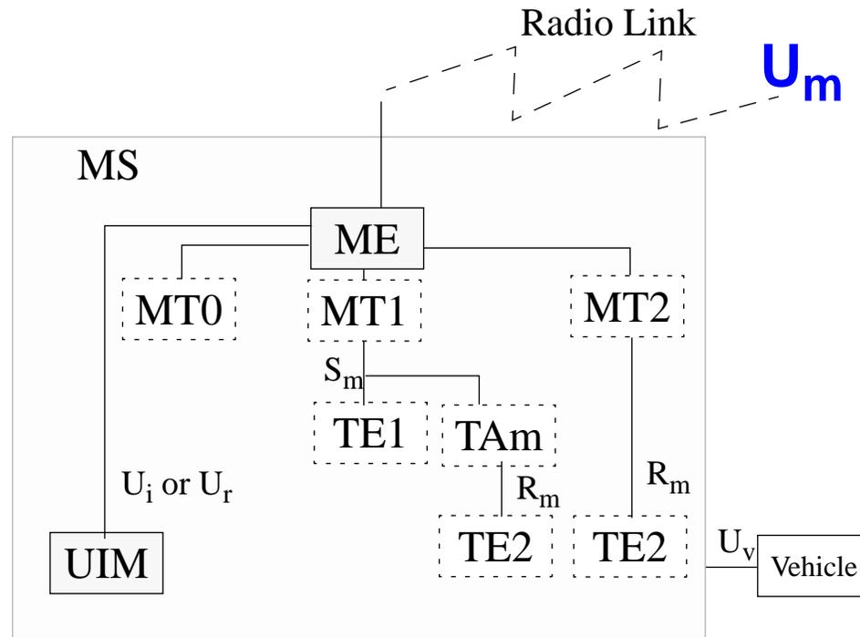
Figure 34: 3GPP2 Architecture (the mobile)
