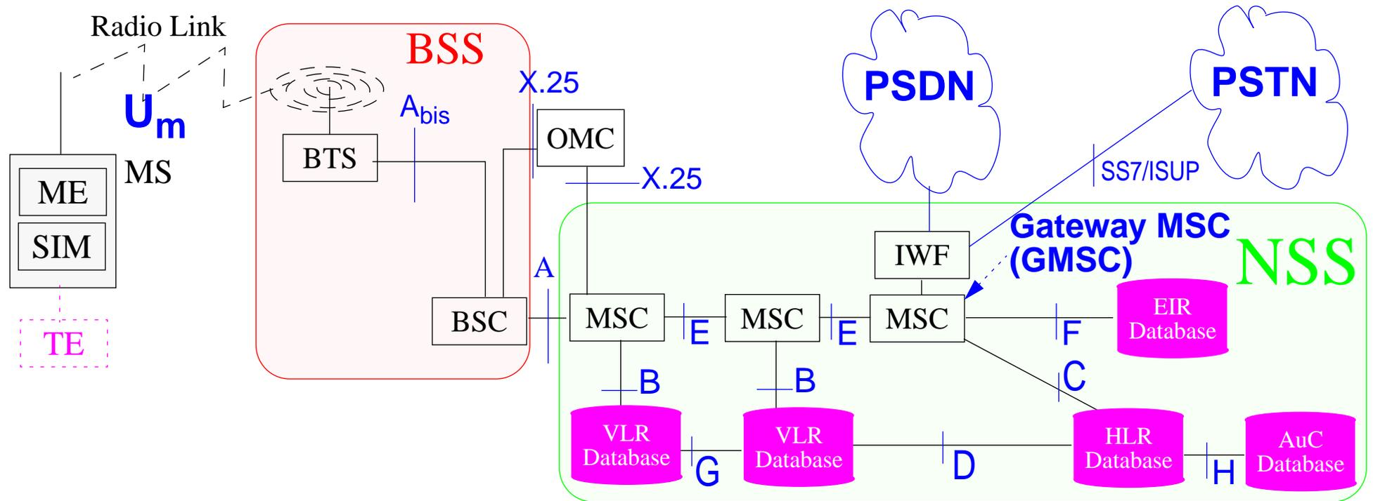
Figure 21: GSM Architecture
