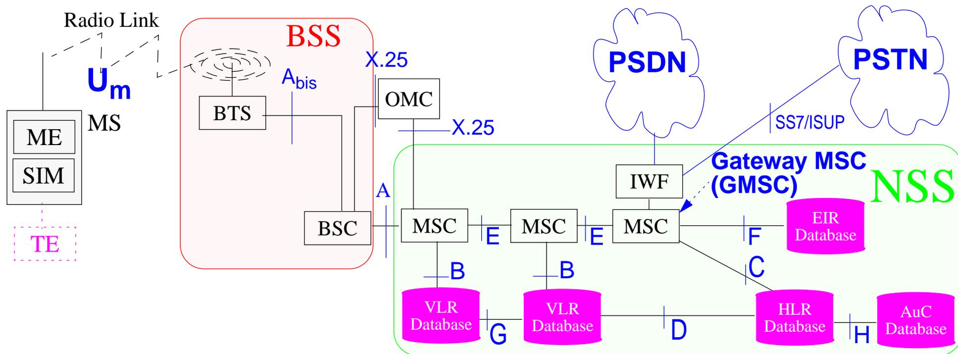
Figure 23: GSM Architecture
