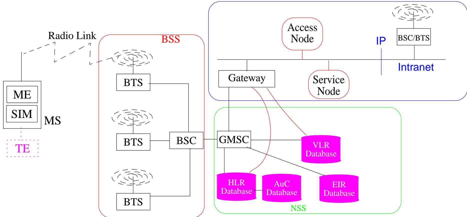
Figure 28: Ericsson's GSM on the Net Architecture
