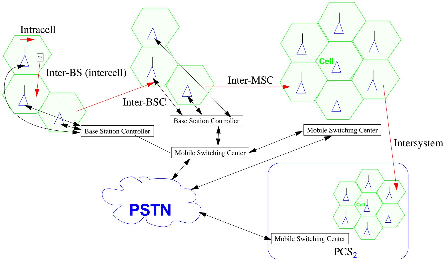
Figure 13: Handoffs, mobile moves within PCS<sub>1</sub> and then on to PCS<sub>2</sub>
