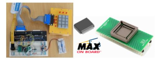
Lab task is to construct a code lock that opens to a unique four-digit code, but we begin by studying a simpler template program, a code lock that opens to one key!
