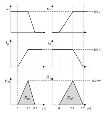
The switching energies at turn-ON and turn-OFF are found to be:
