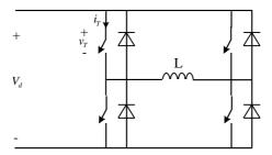
4. Two three-phase thyristor bridge converters are connected to the same grid, 3×400V (line-line), 50 Hz. One converter is feeding 20 kW to a motor at an armature voltage of 200V. The other converter is feeding 500 A to a very large inductance. The direct voltage of the second converter is almost zero. Calculate the total active and reactive power drawn from the grid.
