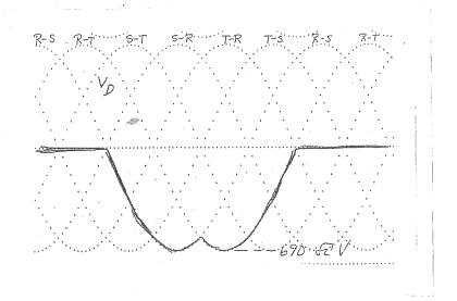
3. The same rectifier feeds a load consisting of a voltage source E in series with a resistance R and an inductance. Calculate  $I_d$  if the line-to-line voltage of the grid is 690 V, E = 690 V and  $R = 24,15 \Omega$ .
