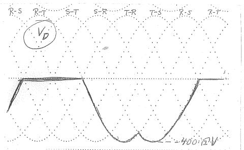
3. The same rectifier feeds a load consisting of a voltage source E in series with a resistance R and a large inductance. Calculate  $I_d$  if the line-to-line voltage of the grid is 400 V, E = 400 V and  $R = 14 \Omega$ .
