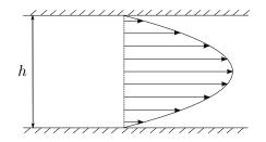
Hint: Assume that the flow is fully developed, meaning  $\frac{\partial}{\partial x} = 0$  for all velocity components. Task 3
