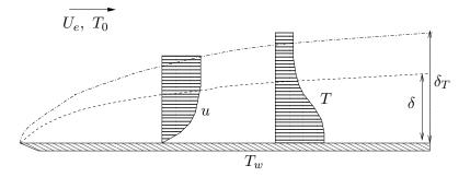
Consider the incompressible flow with free-stream velocity  $U_e$  over a semi-infinite flat plate. Let the incoming flow have a temperature  $T_0$  while the plate is kept at a higher temperature  $T_w$ . The temperature field around the plate obeys the equation
