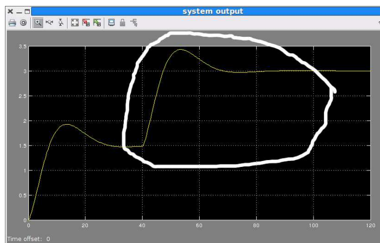
Figure 4: Step response in Simulink model. We are interested in the second step, from 1.5V to 3V
