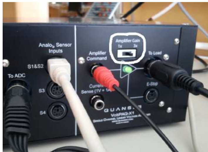
Figure 7: Amplifier Gain should be set to 3x .
