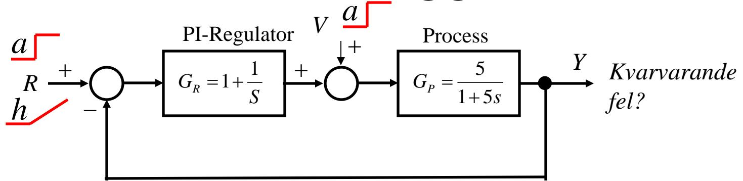
$$\frac{Y}{R} \quad e_0 = ? \quad \frac{Y}{R} \quad e_1 = ? \quad \frac{Y}{V} \quad e_V = ?$$
