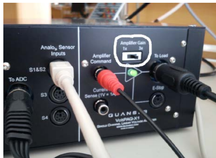
Figure 7: Amplifier Gain should be set to 3x .
