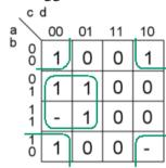
$$y = f(a,b,c)_{\min} = b\overline{c} + \overline{b}\overline{d}$$
