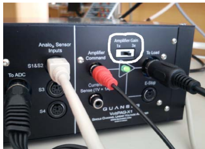
Figure 7: Amplifier Gain should be set to 3x.
