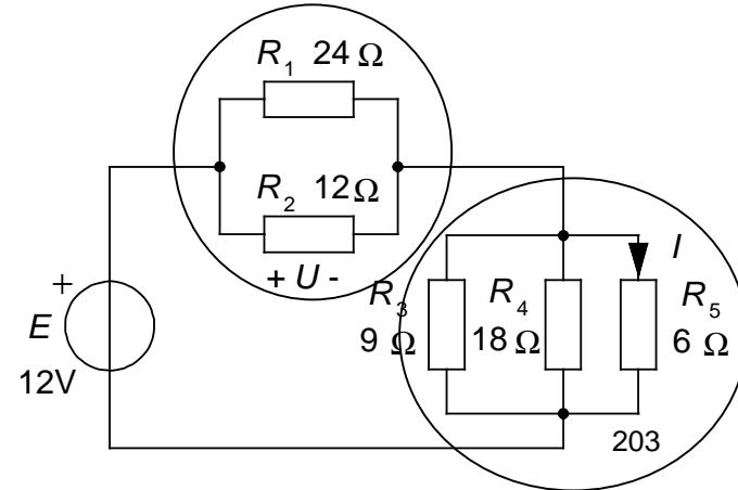
$$R_{1//2} = \frac{24 \cdot 12}{24+12} = 8 \quad \frac{1}{R_{3//4//5}} = \frac{1}{9} + \frac{1}{18} + \frac{1}{6} = \frac{2+1+3}{18} = \frac{6}{18} \Rightarrow R_{3//4//5} = \frac{18}{6} = 3$$
