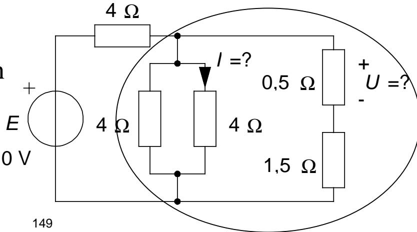
Calculate voltage over the equivalent resistor  $U_{\text{RERS}}$
