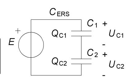
No current/charge can pass through a capacitor. Two series-connected capacitors must therefore always have the same charge!  $Q_{C1} = Q_{C2}$ .
