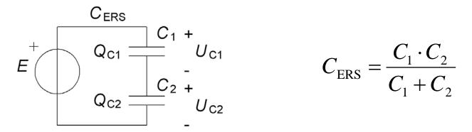
Parallel coupling formula for resistors is comparable to series coupling capacitors formula!
