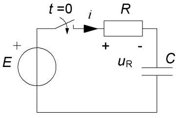
The voltage across the capacitor orginates from the collected charge.
