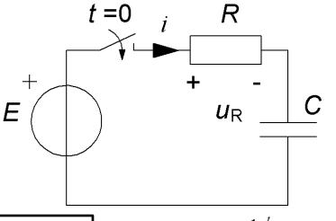
The voltage across the capacitor orginates from the collected charge.
