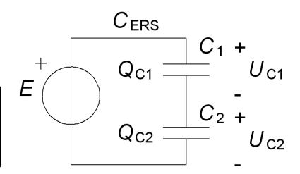
No current/charge can pass through a capacitor. Two series-connected capacitors must therefore always have the same charge!  $Q_{C1} = Q_{C2}$ .
