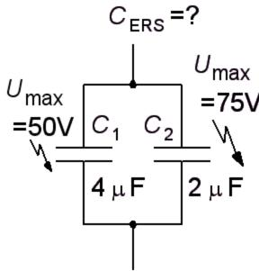
Capacitance is added, the parallel connection is the same as if plate surfaces were added. The capacitor with the worst withstanding voltage determines the equivalent capacitor rated voltage. It is in this capacitor the impact would occur.
