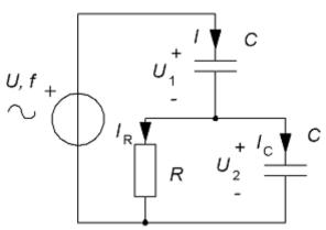
$$U = 20 \text{ V } C = 320 \text{ } \mu\text{F} \quad R = 10 \text{ } \Omega \quad f = 50 \text{ Hz}$$
