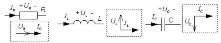
At a certain frequency f the capacitor has the reactance  $|X_C|$  and the resistor R has the same amount (absolute value),  $R[\Omega]$ .
