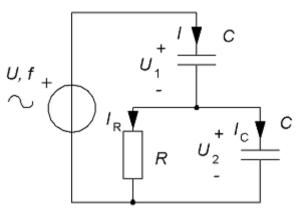
$$U = 20 \text{ V } C = 320 \text{ } \mu\text{F} R = 10 \text{ } \Omega f = 50 \text{ Hz}$$
