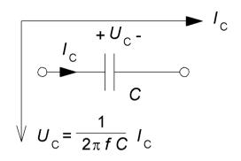
Phasor  $U_C$  is  $I_C/(\omega C)$  and it lags 90° after  $I_C$ . The entity  $1/(\omega C)$  is the "amount" of the capacitor's AC resistance, reactance  $X_C$  [ $\Omega$ ].
