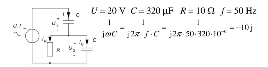
$$U = 20 \text{ V} \quad C = 320 \text{ } \mu\text{F} \quad R = 10 \text{ } \Omega \quad f = 50 \text{ Hz}$$
