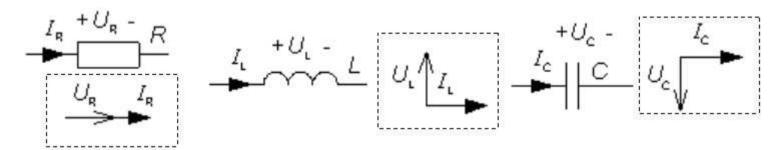
In order to calculate the AC resistance, the impedance, Z, of a composite circuit one must add currents and voltages phasors to obtain the total current I and the total voltage U.
