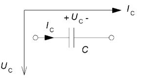
The method with complex pointer *automatically* keeps track of the phase angles if we consider the capacitor reactance  $X_{\mathbf{C}}$ as **negative**, and hence the inductor reactance  $X_{\mathbf{L}}$  as **positive**.
