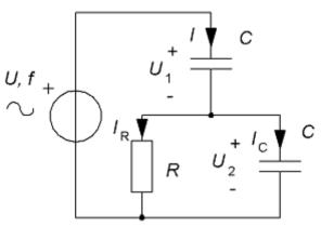
$$U = 20 \text{ V } C = 320 \text{ } \mu\text{F } R = 10 \text{ } \Omega \text{ } f = 50 \text{ Hz}$$
