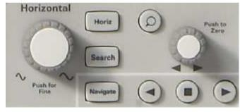
With the "Magnifierbutton" you can select a part of the trace to study in detail.
