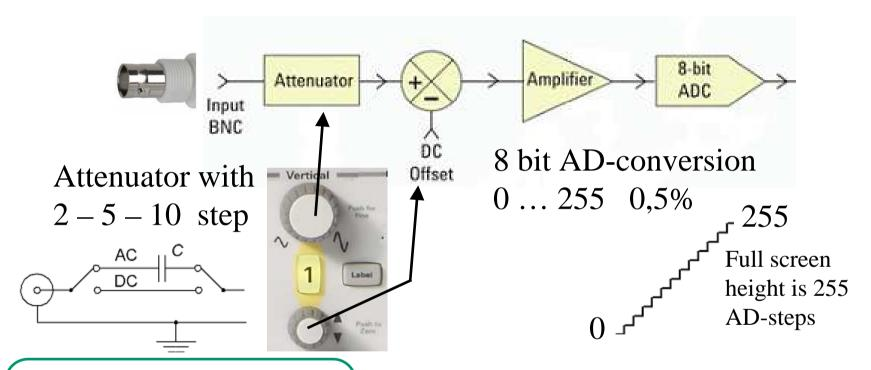
Input could be AC-coupled in order to block DC-components. **DC-coupled is the default setting**.
