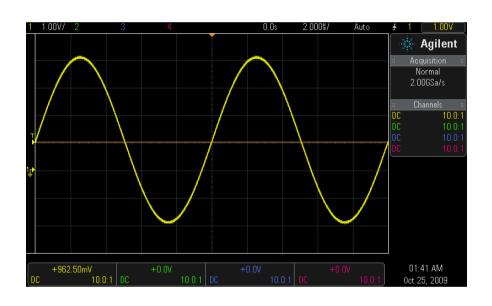
With the timebase system you change the samplingfrequency for the data acquistion, and choose what part of the stored signal to display.
