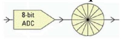
Data is continuously stored in a circular buffer.
