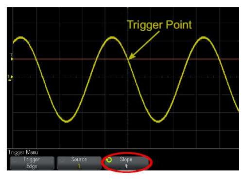
Trigger-point **level**, and **slope** (slope), could be choosen arbitrary.
