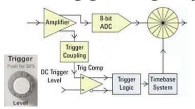
When buffer content is shown continuously in sequence on the screen, it has to be synchronized in order to give a stable trace.
