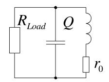
If the loaded resonance circuit is to become the wanted Q value one has to have an inductor with a much better  $Q_0$ !
