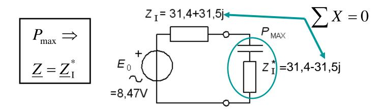
At power match with a load equal to the complex conjugate of the internal impedance, the effect:
