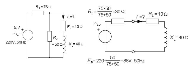
The emf and resistors – this time as with DC circuits ...
