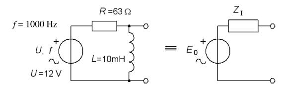
$E_0$  is calculated as the divided voltage. If U is the reference phase we get  $E_0$  8,47 V and gets the phase 45° to U. If there are no other voltage sources or current sources in the circuit then we don't have to keep track on the phase, as  $E_0$  might as well become the network's new reference phase!
