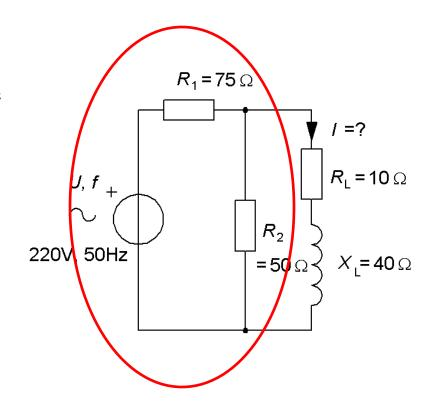
Calculate the Thevenin equivalent  $E_0$  and  $R_{\rm I}$  of this circuit.
