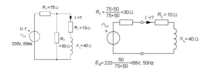
Calculate the Thevenin 0, f this equivalent  $E_0$  and  $R_{\rm I}$  of this circuit.
