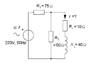
Calculate the Thevenin equivalent  $E_0$  and  $R_I$  of this circuit.
