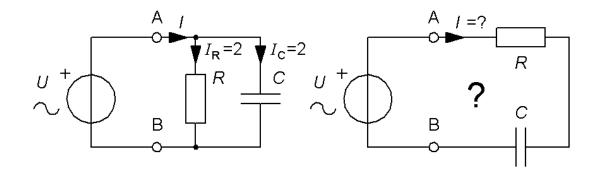
When a resistor R and a capacitor C is connected in parallel to a voltage source U each of them get the current 2A.
