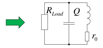
• When the circuit is loaded with  $R_{\text{Load}}$  the Q-value will change from  $Q_0$  to Q!
