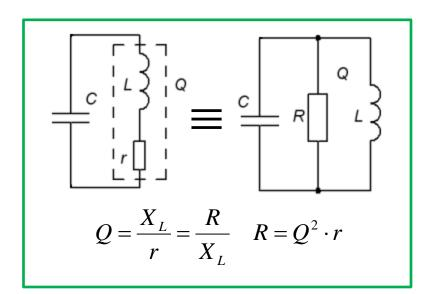
Usually the resonance circuit is loaded!
