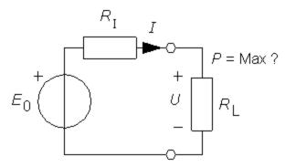
$$\frac{1}{P} = \frac{1}{E_0^2} \cdot (\frac{R_L^2}{R_L} + \frac{R_I^2}{R_L} + 2 \cdot \frac{R_I \cdot R_L}{R_L}) = \frac{1}{E_0^2} \cdot (R_L + 2 \cdot R_I + \frac{R_I^2}{R_L})$$
