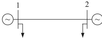
Figure 7.12. Single-line diagram of a balanced two-bus power system.
