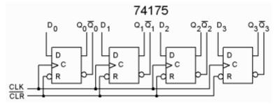
At the lab, we use a compact circuit 74175 with 4 D-flip-flops, where all the flip-flops reset inputs are connected to the same pin. It is easy to reset the flip-flops, but how does one go about to set them to any value? At the lab, you will learn how to do this by connecting them as a PRBS generator.
