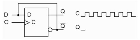
What happens to a D-flip-flop that has its D input connected to its inverted output?
