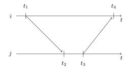
$t_2 = t_1 + D + \delta + n_2$  $t_4 = t_3 + D - \delta + n_4$
