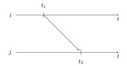
$$\begin{array}{l} c_{i}\left(t_{1}\right)=t_{1}+n_{1}\\ c_{j}\left(t_{2}\right)=t_{2}=t_{1}+D+\delta+n_{2}\\ & \uparrow & \swarrow\\ & \text{propagation}\\ & \text{delay} \end{array}$$
