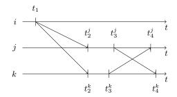
$t_{4}^{k} = t_{3}^{j} + \delta_{jk} + n_{4}^{k}$   $t_{3}^{j} = t_{2}^{j} + \Delta_{j} = t_{1} + \delta_{ij} + \Delta_{j} + n_{3}^{j}$   $t_{4}^{j} = t_{3}^{k} + \delta_{kj} + n_{4}^{j}$  $t_{3}^{k} = t_{2}^{k} + \Delta_{k} = t_{1} + \delta_{ik} + \Delta_{k} + n_{3}^{k}$
