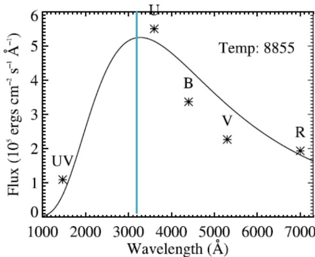
The maximum flux corresponds to a wavelength of  $3200 \text{ \AA} = 320 \text{ nm}$ . Wine's displacement law gives
