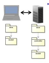
The MVVM pattern intoduces a client-side model which reflects the server-side model and is responsible for notifying the view of updates. DOM
