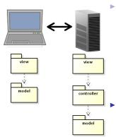
The MVVM pattern intoduces a client-side model which reflects the server-side model and is responsible for notifying the view of updates.
