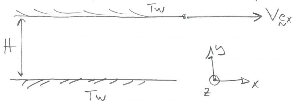
Both plates have the same temperature,  $T_w$ , but different velocities according to the figure.
