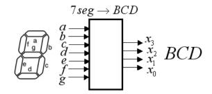
a) (1p) Set up the **truth table** for the ten BCD numbers. Black segment in figure is "1".  $(x_3x_2x_1x_0)_{RCD} = f(abcdefg)$
