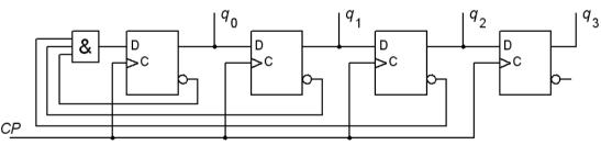
**a**) (2p) Analyze the sequential circuits in the figure and draw the **full state diagram** and the **full state table**. If the counter would start in any other state than any of the four desired "one hot" states, how many clock pulses are required, in the worst case, before the counter has "corrected" this and ends up in the correct sequence?
