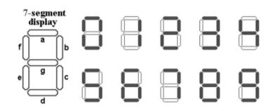
c) (2p) Draw the karnaugh maps for the four BCD-code bits and derive the **minimized expressions** for  $x_3$   $x_2$   $x_1$   $x_0$  in SoP-form. Segment combinations that never occurs should be exploited as don't care. (With the excluded segments in the truth table, the number of variables will be manageable).
