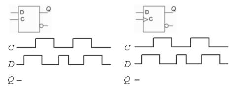
Complete the timing diagrams for the D-latch and D-flipflop by drawing signal Q for booth cases. Draw the figure so that it is clear **what** is causing the changes in the Q!
