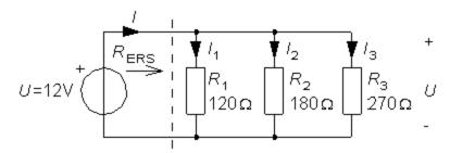
From the emf U one only sees the current I, it could likely go to a lonely resistor, an equivalent resistance  $R_{\text{ERS}}$ . Ohms law gives:
