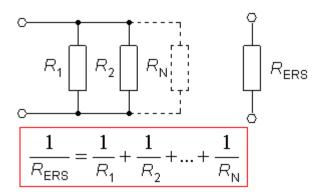
Parallel connected components, are characterized in that they have **both connections** in common with each other.
