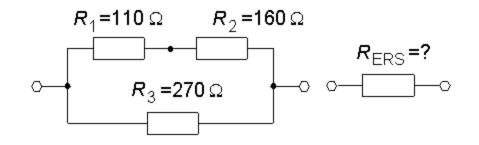
$$R_{ERS} = \frac{R_3 \cdot (R_1 + R_2)}{R_1 + R_2 + R_3} = \frac{270 \cdot (110 + 160)}{110 + 160 + 270} = 135 \,\Omega$$
