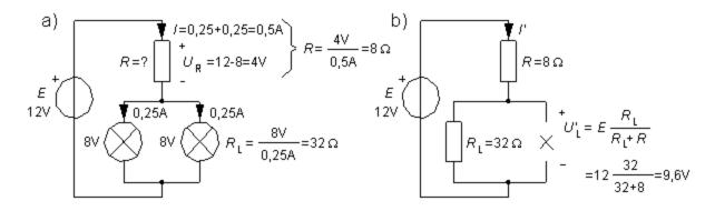
b) Suppose that one of the lamps breaks – how big will then the voltage over the other lamp be?
