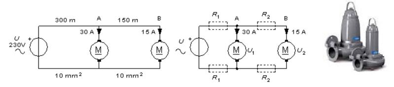
Two electric pumps A and B are placed 150 m from each other. A and then B, are powered by 230V from a socket 300 m away. A pump draws the current 30 A and B 15 A. See figure.
