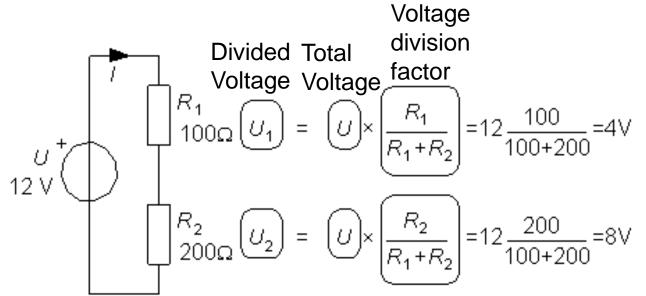
According to the voltage divider formula you get a divided voltage, for example  $U_1$  across the resistor  $R_{1,}$  by multiplying the total voltage U with a voltage division factor. This voltage division factor is the resistance  $R_1$  divided by the sum of all the resistors that are in the series connection.
