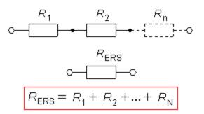
Series-connected components, are characterized in that they are interconnected in **one** point.
