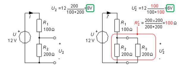
For a voltage divider to maintain it's divided voltage when it is loaded, it is required that the connected load has a much higher resistance than the resistors included in the voltage divider.
