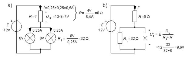
a) Calculate the series resistor R so that the lamp voltage will be correct, 8 V.
