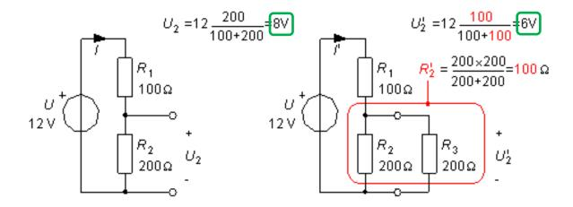
In the figure above to right, the resistor  $R_3 = 200 \Omega$  symbolizes the electronic equipment.
