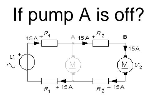
How big will the voltage be at pump B,  $U'_2$ , when pump A is off?
