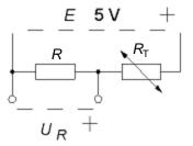
If a fixed resistor R is connected in series with the NTC thermistor  $R_T$  this combination will have a lesser nonlinearity than the thermistor alone. We will let the two resistors form a voltage divider.
