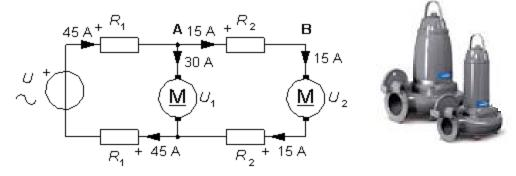
$U_1 = U - 2 \times R_1 \times 45 = 230 - 2 \times 0,54 \times 45 = 181,4 \text{ V}$
