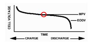
Curve midpoint is called MPV (Midpoint Voltage) and it is this value of voltage that is usually stated as the terminal voltage. The discharge does not necessarily have last for one hour. The discharge time is therefore indicated with the capacity number index.
