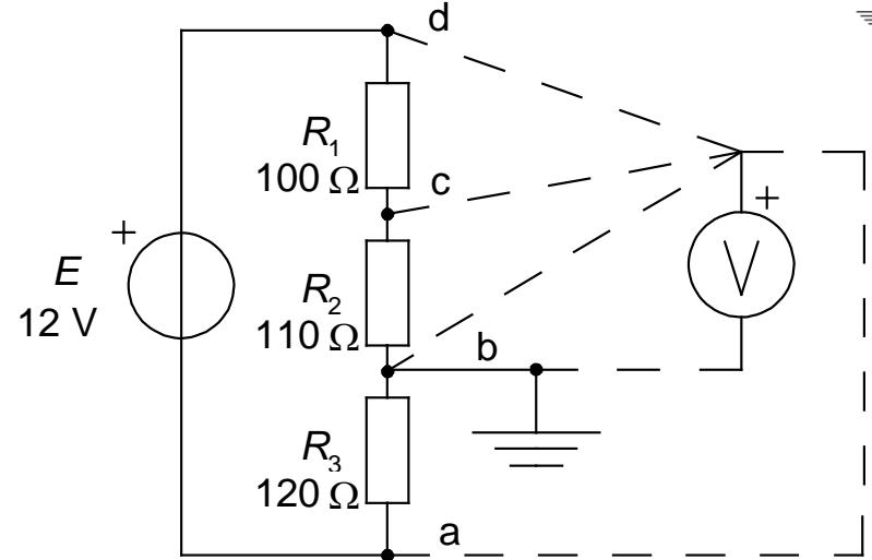
One measures the potential (voltage relative to ground) at various sockets on the the voltage divider.
