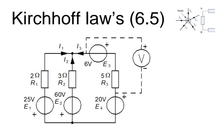
a) Use Kirchhoff's two laws to set up an equation system by which the three currents  $I_1$   $I_2$  and  $I_3$  can be calculated. (You need not solve the system of equations)
