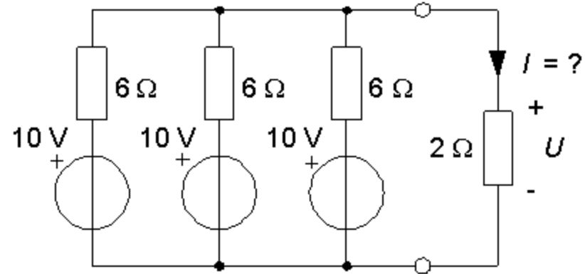
The three internal resistances  $6\Omega$  have common voltage in both ends, and is thereby effectively paralleled.  $R_I = 6/3 = 2\Omega$ .  $I = 2,5 \text{ A}$  och  $U = 5\text{V}$ .
