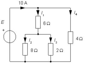
$$R_{ERS} = \frac{\left(6 + \frac{8 \cdot 2}{8 + 2}\right) \cdot 4}{\left(6 + \frac{8 \cdot 2}{8 + 2}\right) + 4} = 2.62 \,\Omega \quad E = R_{ERS} \cdot I = 2,62 \cdot 10 = 26,2 \,\text{V}$$
