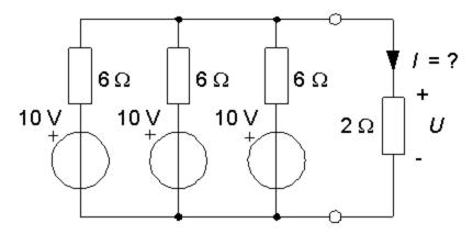
The three internal resistances  $6\Omega$  have common voltage in both ends, and is thereby effectively paralleled.  $R_{\rm I} = 6/3 = 2\Omega$ . I = 2,5 A och U = 5V.
