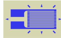
Industrial scales. Two strain gauges on the top of a beam increases from 500 to 501. Two strain gauge on the bottom of a beam decreases 500 to 499.
