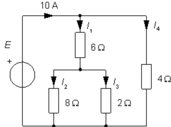
$$R_{EIS} = \frac{\left(6 + \frac{8 \cdot 2}{8+2}\right) \cdot 4}{\left(6 + \frac{8 \cdot 2}{8+2}\right) + 4} = 2,62 \Omega \quad E = R_{EIS} \cdot I = 2,62 \cdot 10 = 26,2 \text{ V}$$
