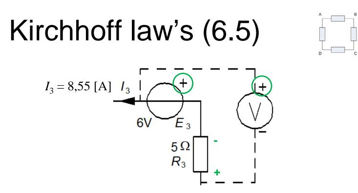
Voltmeter (U) shows  $U + E_3 + R_3 \cdot I_3 = 0 \implies U = -6 - 5 \cdot 8,55 = -48,75 \text{ V}$
