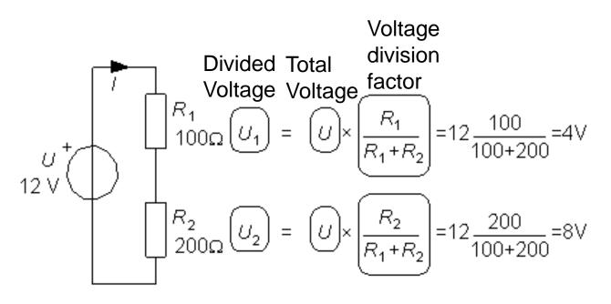
According to the voltage divider formula you get a divided voltage, for example  $U_1$  across the resistor  $R_1$ , by multiplying the total voltage U with a voltage division factor. This voltage division factor is the resistance  $R_1$  divided by the sum of all the resistors that are in the series connection.
