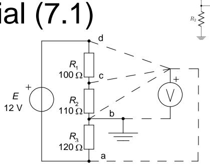
One measures the potential (voltage relative to ground) at various sockets on the the voltage divider.
